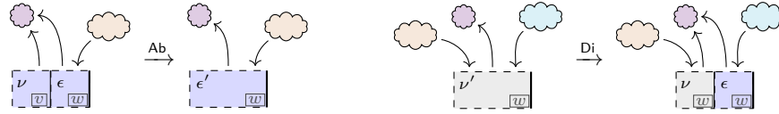
Fig. 7. Schematic depictions of the absorb (left) and dilute (right) rewrite rules, that focus on the segment of the dovetailed messages together with all pointers into and out of them, within a particular memory snapshot. The circular cloud represents the subset of the memory that the messages in focus are pointing to, showing that they all have the same view. The elliptical clouds represent views—including the initial and final view, as well as other messages—that point to each of the dovetailing messages. Left: The message \nu is “absorbed” into the message \epsilon to become \epsilon' . No view may point to \nu . Right: The message \nu' “dilutes” into \nu and \epsilon . While \epsilon must be a local message, \nu and \nu' can appear anywhere the trace’s sequence, as long as they appear in the same places in the sequence, and that \epsilon does not appear before. The views that point to \nu' before diluting can point either to \nu or to \epsilon after diluting.
